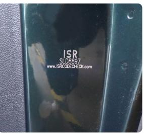
Marking of all types of motor vehicle: In addition to windows, painted metal and plastic component parts can also be marked
